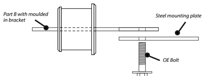
Figure 5 - Fit additional mounting plate if required
